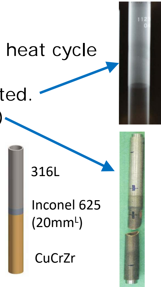
Tensile test specimen (Top: RT image, Right: After fracture)
