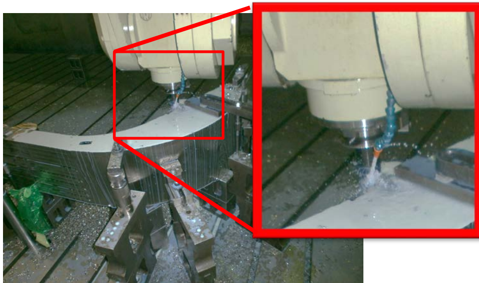
3D machining of SSS with 5-axis machine
